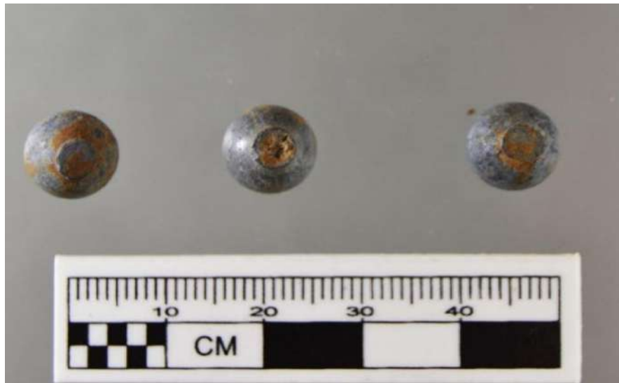
Figure 10. Sprue Shapes, Oval (left), Round (middle and right).
