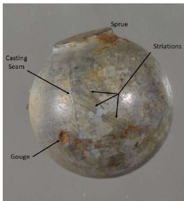
Figure 23. Locus H Musket Ball with Gouges and Striations.
