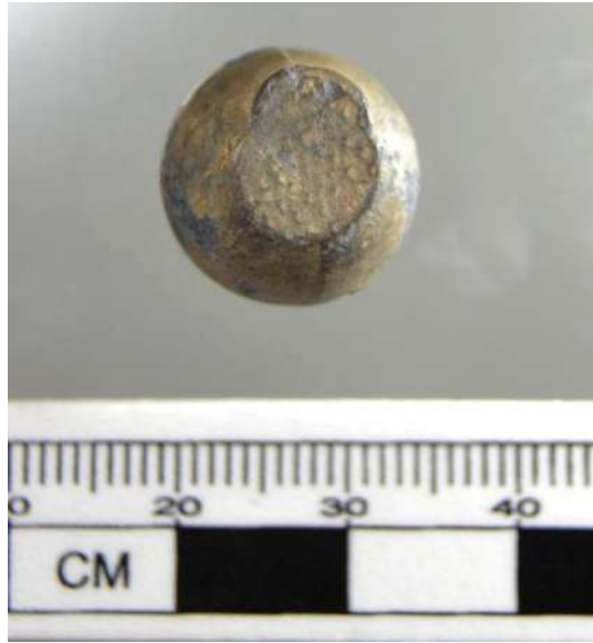
Figure 19. Ramrod Mark with Wadding/Fabric or Thimble Impression.
