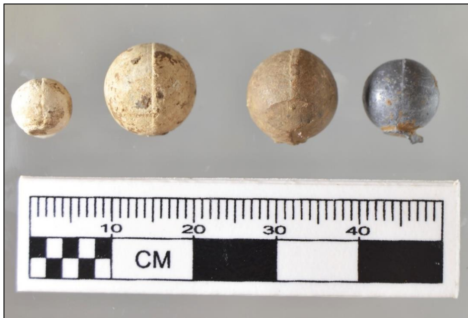
Figure 12. Misaligned Seam (left two); Prominent Seam from spillage (third from left); Normal Seam (far right).
