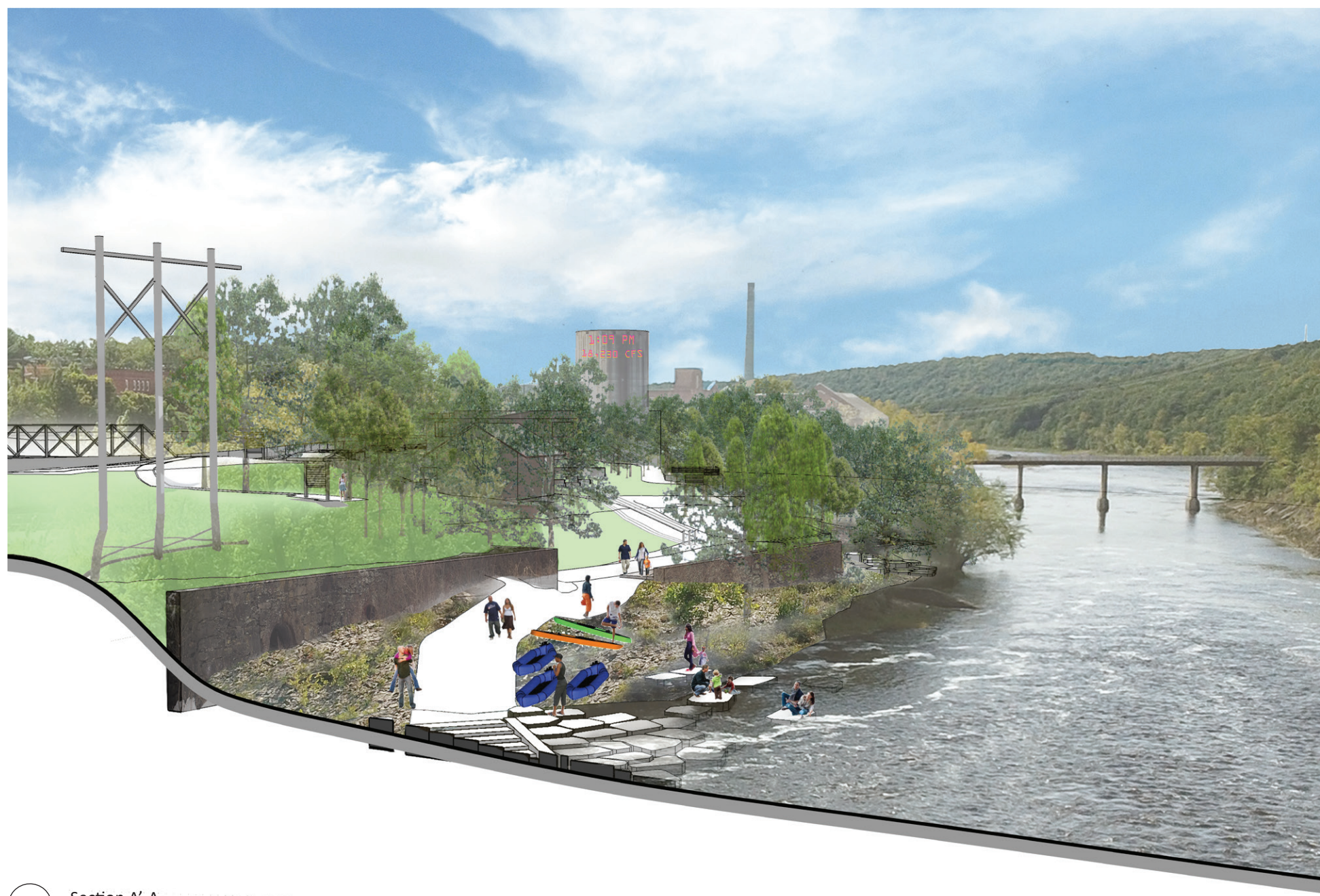
Section A'-A: A section view through the Entry and River Access area showing the primary boat slipway. The slipway is composed of large oxbow boulders that descend into the river allowing visitors to safely access the river at different levels. The slipway gives white water enthusiasts access to the exciting rapids below the Great Falls. The water access at the park allows boaters traveling down the Connecticut River to portage around the dam.
