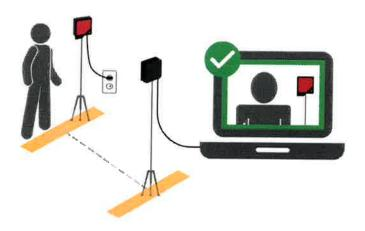
Seek Scan is an infrared thermal imaging system designed to measure human skin temperature. The system will automatically detect a face, measure the person's facial skin temperature and display an alert if they are above or below the customizable alarm temperature. Set up in minutes with two tripods and a Windows PC.
