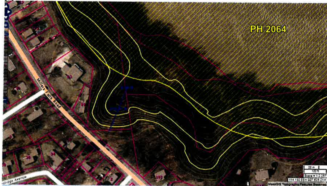
Image 2: Project area with 3 meter contours. Blue line is approximate storm water conveyance pipe.
