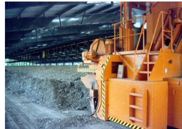
Floor aerated windrow
